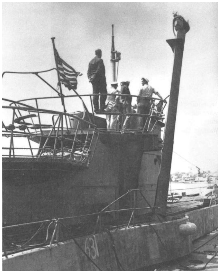
Using the snorkel mast, shown here next to the conning tower, U-boats could run their diesel engines while submerged by sucking air through an intake at the top of the mast while blowing diesel fumes out of the snorkel's exhaust manifold. (U.S. Navy Photo)
